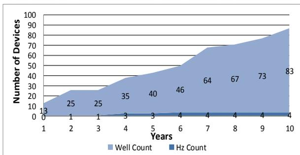
The collected data points shown were gathered over a period of ten (10) years and through multiple phases of gas well construction. Average gas flow rates for both horizontal and vertical gas wells were totaled each year to determine a total average system flow rate for the site. Gas production by year is shown on Figure 5.
