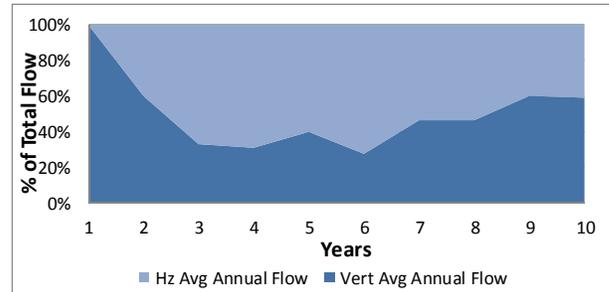
Although gas collection rates observed from the horizontal gas wells declined following installation of the vertical gas wells, the data shows that these wells are still effectively capturing a significant volume of gas. At year 10, three years after the last horizontal installation, the horizontal gas wells continue to collect nearly 41% of the total site gas flow at the site.
