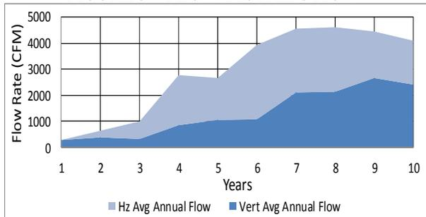
Horizontal gas wells have the capacity to collect a greater volume of gas than vertical gas wells due to their size resulting in a larger area of influence. On average, gas volumes collected from horizontal gas wells for the study site represents 49.7% of the total gas flow over the ten year period. The percentage of total site LFG flow
