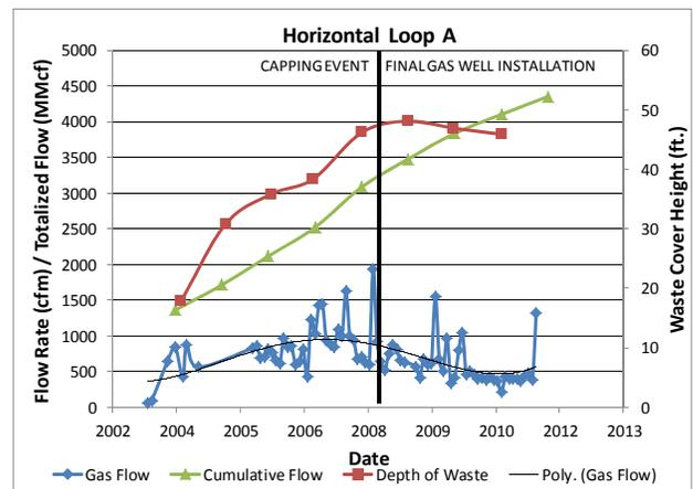
Data plotted for Loop A demonstrates significant long-term gas production and collection over an 8-year period. Gas collection rates generally increased over time up until final grades were reached and the final capping and vertical wells are installed. Gas collection rates generally decreased after the capping event; however, the horizontal remained very productive. The site was able to collect gas from the active area as filling operations
